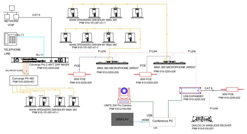
NOTE: ANY INDIVIDUAL P-LINK MUST NOT EXCEED 200 FEET / 61 METER IN LENGTH
